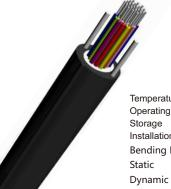
Temperature Range Operating : -40°C to +70°C Storage : -50°C to +70°C Installation : -30°C to +70°C Bending Radius: Static 10D Dynamic 20D
